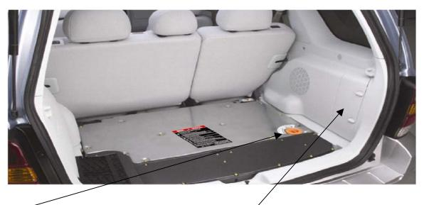
High Voltage Service Disconnect Switch panel
